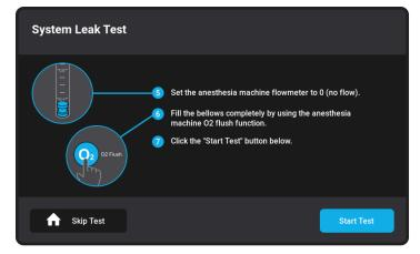
Once these steps are completed, press "Start Test," and the leak test will automatically begin.
