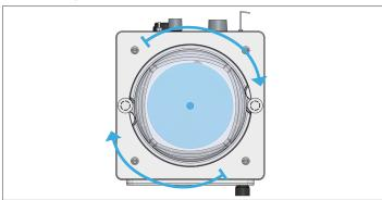
Reassemble the bellows and the bellows housing on the ventilator.
