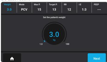
You can access your last patient's parameters by pressing the last patient button located at the bottom left of the ventilator screen. This feature is particularly useful in case of a momentary power outage. Instead of re-entering your last parameters, you can simply select the last patient to regain access to their information.
