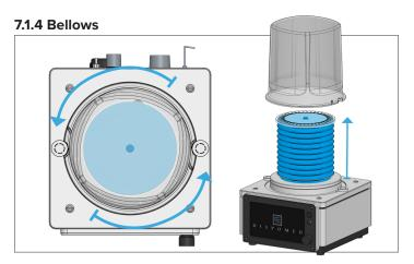
Remove the bellows housing and then carefully remove the silicone bellows from the ventilator.
